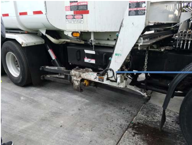
Graphic 2: Residential Recycling Automated Side Loader Arm
