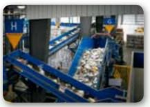
The MRF includes separate tipping areas for residential and commercial recyclables, which are then processed using a series of conveyors, screens, magnets and optical sorters to separate paper from containers. These materials are then further separated into newspaper, mixed paper, cardboard, glass, aluminum, tin and plastics. The MRF equipment does the bulk of the materials separation, while the sort-line workers remove non-acceptable items from the separated recyclables.
